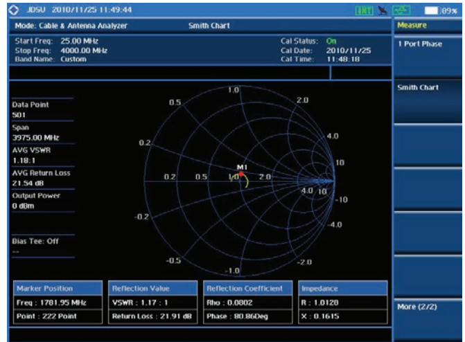
Cable and antenna test — Smith Chart
