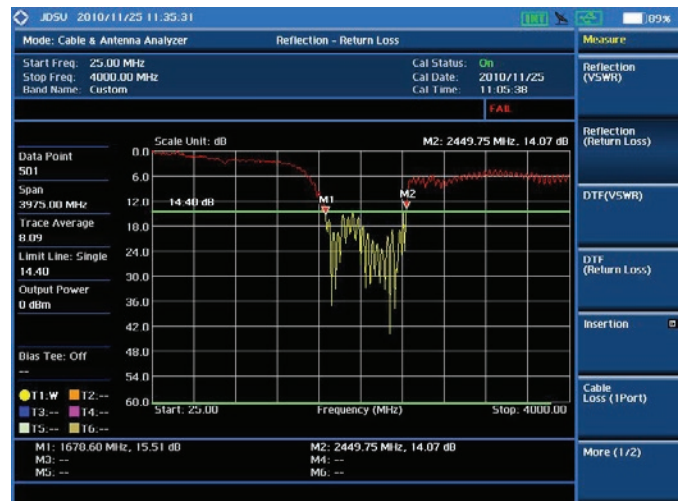
Cable and antenna test — Reflection
