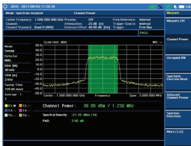
RF test — Channel Power
