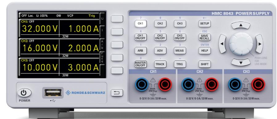
All connectors, including SENSE, are available on the rear panel. A cage clamp facilitates rack installation and deinstallation. The LXI-compliant power supply can be controlled via LAN, USB or an optional GPIB interface. The CDC (virtual COM port) and TMC classes are supported for communications via USB. The remote control commands are based on the SCPI standard.
