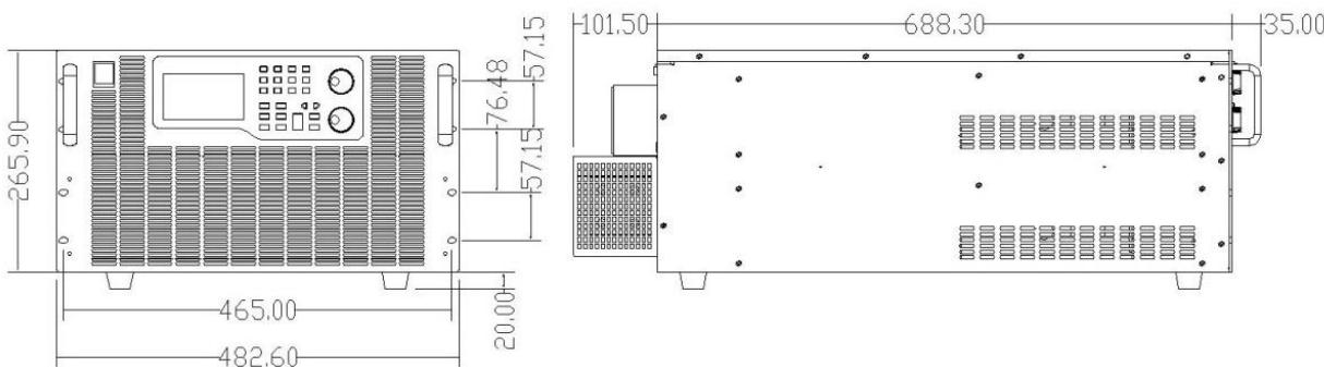
20kW~30kW model dimension (models with voltage &gt; 40V)
