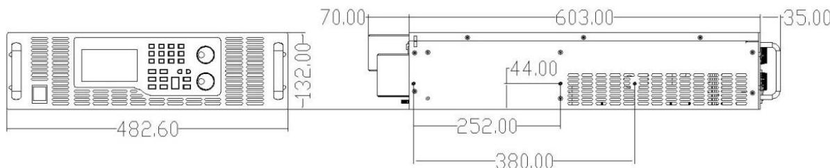
20kW~30kW model dimension (models of 40V or below)
