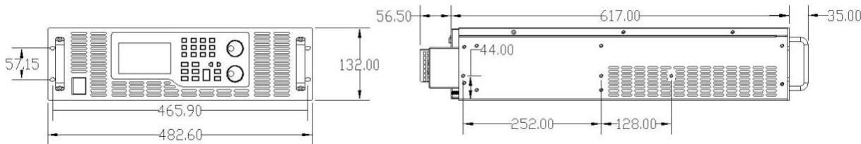
5kW~15kW model dimension (models with voltage &gt; 40V)
