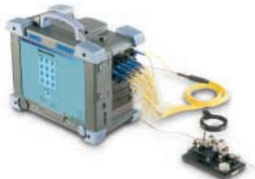
The FTB-400 configured as a ribbon test kit for OTDR testing in a high-fiber-count environment.
