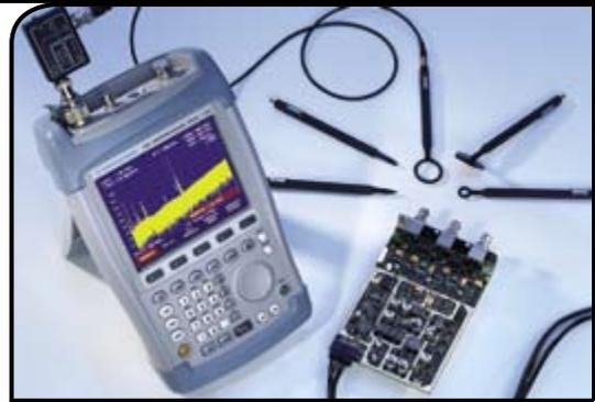
R&S®FSH with near-field probe set and DUT
