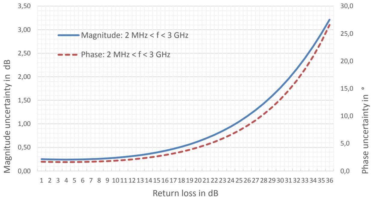
Uncertainty of reflection measurements with the R&S®ZN-Z103 calibration unit;
