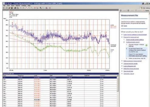
Preview measurement (Pk and Avg) with determination of the local maxima (here, 25 subranges) for subsequent final measurement (QP and C-Avg).
