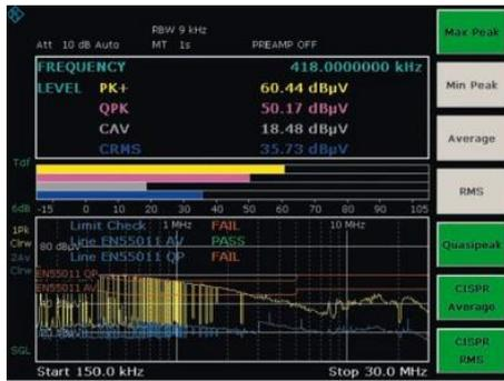
Menu for selecting weighting detectors. Values produced by a maximum of four different detectors are simultaneously displayed, both numerically and as an analog bargraph.
