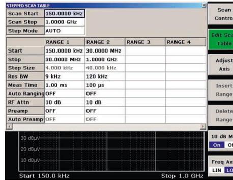
In receiver mode, the R&S®ESL is tuned in fixed frequency steps in accordance with the settings in the SCAN table. The SCAN table can be programmed for a maximum of ten frequency subranges with independently selectable parameters.
