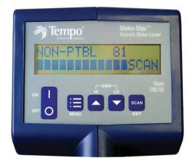
Scan Mode: Automatically determines marker type detected (power, water, sanitary, telephone, gas, CATV, non-potable)
