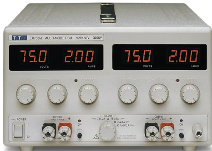
As a dual, each output provides 0 to 75V at 0 to 2A (mode A). As a single, the output can be selected as either 0 to 75V at 0 to 4A (mode B) or 0 to 150V at 0 to 2A (mode C). In single modes, the unused half of the unit becomes completely inoperative and its displays are blanked.
