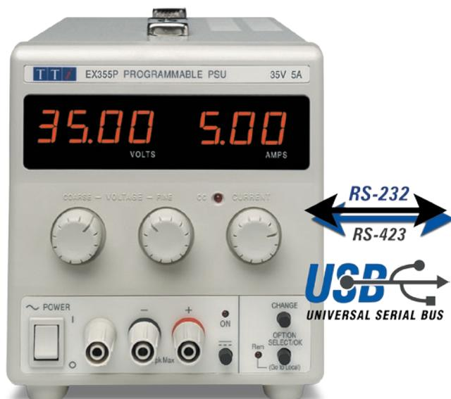
A simple command set allows remote control of voltage, current and output enable together with read-back of metering values and operational status. Local control is via three rotary encoders providing rapid and accurate setting of voltage and current during bench use.
