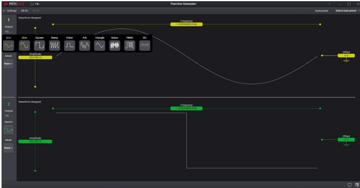
Figure 5. Select and configure your required waveform
