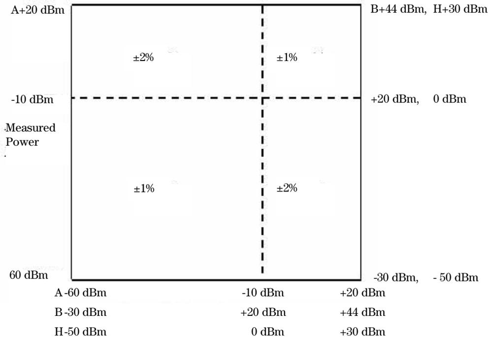
Figure 2 shows the typical uncertainty in making a relative power measurement, using the same power meter channel and same power sensor to obtain the reference and the measured values, and assumes that negligible change in frequency and mismatch error occur when transitioning from the power level used as the reference to the power level being measured.
