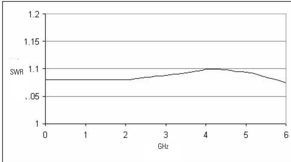
*Typical SWR, 10 MHz to 18 GHz, (25 °C ± 10 °C) for E9300B and E9301B sensors*
