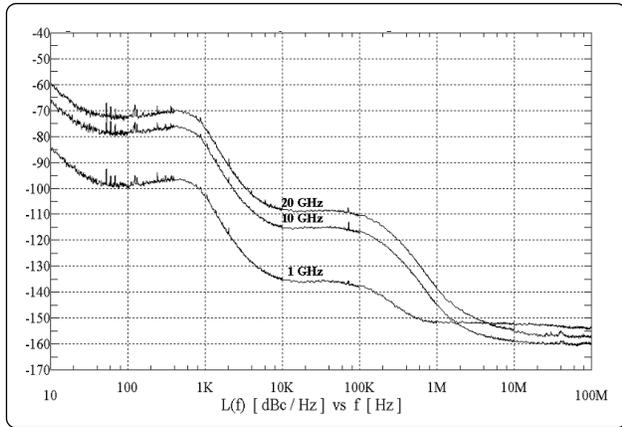
**Standard phase noise performance with I/Q modulation on<sup>1</sup>**
