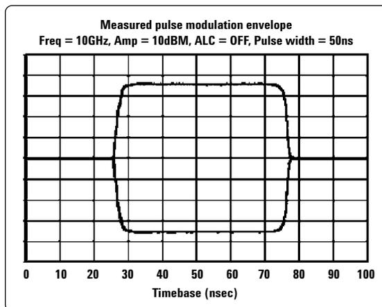
1. With ALC off, specs apply after the execution of power search. Specs apply with Atten Hold off (default mode), or ALC level between 0 and +10 dBm.
