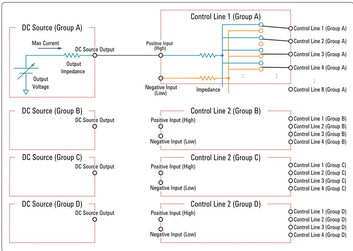
Figure 3-7. Control line pin assignment (E5092A-020)
