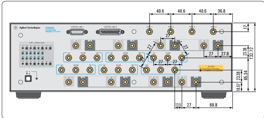
Figure 3-3. Dimensions (rear view, with Option E5092A-020, in millimeters, nominal)
