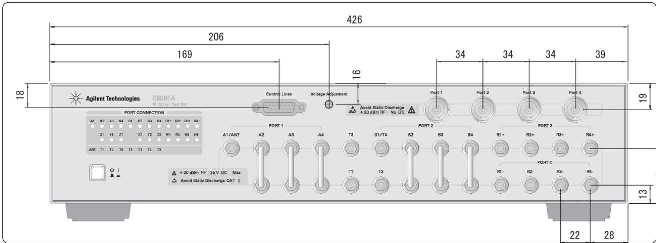
Figure 2-3. Dimensions (rear view, in millimeters, nominal)
