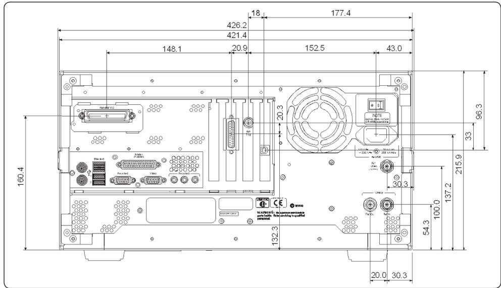
**Figure 1-3. Dimensions (side view, in millimeters, nominal)**
