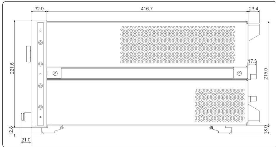
**Figure 1-4. Dimensions (top view, in millimeters, nominal)**
