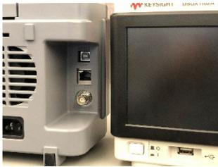
Built-in USB host and USB device ports make PC connectivity easy. BenchVue Software with the BV0004B BenchVue Oscilloscope app (standard) lets you control and visualize the 1000 X-Series and multiple measurements simultaneously. Build automated test sequences just as easy as using your front panel. Save time with the ability to export measurement data to Excel, Word, and MATLAB in three clicks. Monitor and control your 1000 X-Series with a mobile device from anywhere.
