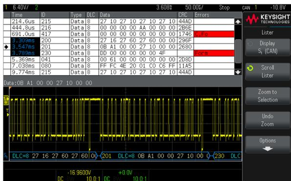
The 1000 X-Series is a powerful protocol analyzer that enables hardware-based specialized serial communication analysis (standard). Other vendors' oscilloscopes use software post-processing techniques that slow down the waveform and decode update rate, but the 1000 X-Series has faster decoding based on hardware technology that enhances scope usability and the probability of capturing infrequent serial communication errors.
