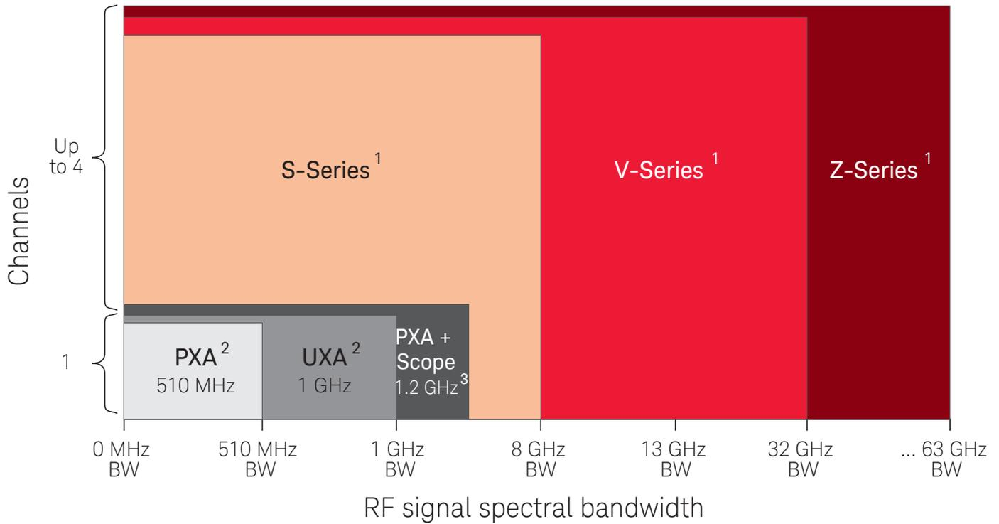
1. S, V, and Z-Series 2 ch full bandwidth, 4 ch half bandwidth.
