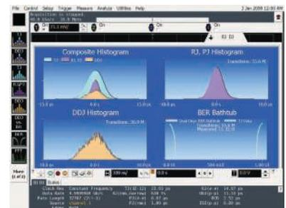
Analyze jitter plus RJ/DJ separation.
