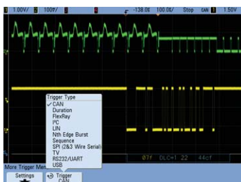
Trigger on and decode CAN serial packets.
