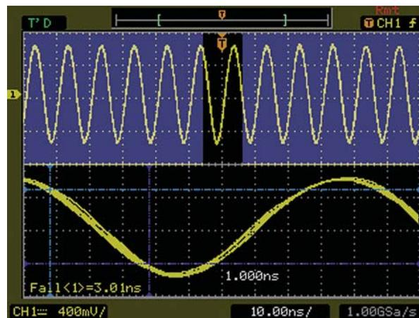
**Figure 2.** Want to see the big picture but still get all the details? Use the delayed sweep mode to zoom in on a particular area of interest on your signal while still viewing the entire captured waveform.
