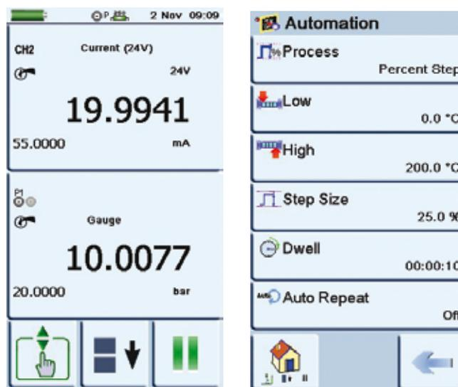
The DPI 620 includes comprehensive documenting features for automating instrument calibration when used in conjunction with Intecal Calibration Management software.
