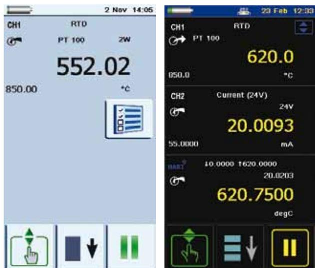
configured to show up to six reading windows and can show electrical and temperature inputs and outputs, two pressure module readings, an IDOS pressure measurement, and a USB-connected device, as well as a HART summary window or full HART communicator with active mA measurement and actual primary variable readings.
