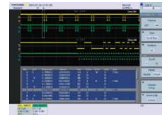
Example of I 2 C Bus Analysis Display
