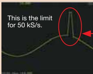
The waveform shown above was captured at a sampling rate of 50 kS/s. The occurrence of noise can be confirmed in the graph, but the time resolution is too low to capture the waveform accurately.
