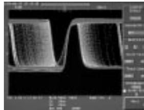
In addition to a persistence display which accumulates data in monochrome, the DL7100 has a color accumulate mode that distinguishes the frequency of events by color. This is useful for jitter evaluation and identifying abnormal signals.
