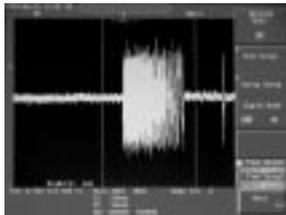
Count the number of pulses in a waveform between cursors. This is useful for counting the pulses of a stepping motor, the rack error signals on an optical disk, or interrupt signals due to software debugging.
