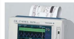
By simply pressing IMAGE SAVE key, you can easily and quickly save screen image data to the PC card, USB flash memory, MO, or USB hard disk media. Screen image formats include BMP, TIFF, PS, PNG, or JPEG. Thumbnail images make previewing your captured images simple. The thumbnail appears together with the file name, allowing you to confirm, delete, or make spot changes to the image file name.
