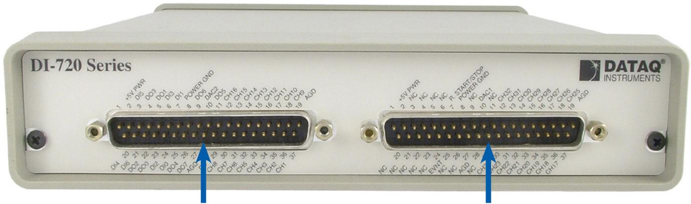
Access to channels 1 through 16 and I/O accessories via 37-pin D type, male connector.
