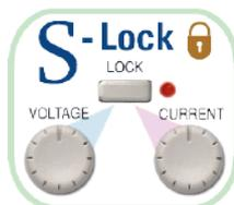
The main disadvantage of analog controls is stability and security. The settings of analog potentiometers can drift over time. More importantly, the settings can be changed accidentally with potentially serious consequences.
