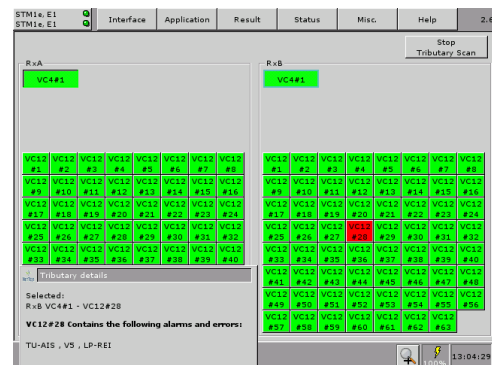
Fig. 19: The tributary scan feature gives you a quick overview of the tributaries of the monitored line with color identification of problems.
