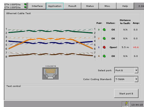
Fig. 13 The CMA 3000s cable test facility makes it easy to identify failures on electrical cables like short circuits or breaks of a wire pair. The cable test facility also indicates the distance from the instrument to the fault.
