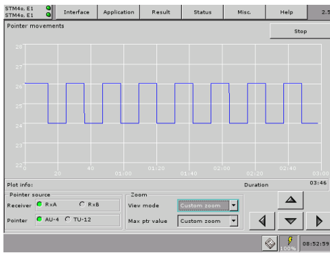
Fig. 20 The pointer graph allows a detailed analysis of pointer movements in the monitored SDH signal.
