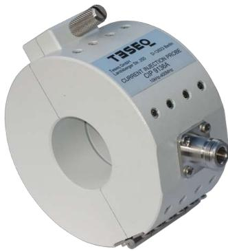
The CIP 9136 probe has been manufactured to drawings and specifications laid down by QinetiQ. It meets the requirements for HIRF testing where conventional ferrite core material cannot handle the higher powers required (up to 1000 W), without changing characteristics when heated. Whilst having been initially designed to meet the specific requirements of Aircraft Testing from 10 kHz to 50 MHz, the CIP 9136's unique non-ferrite core allows wide band performance from 10 kHz - 400 MHz, and above.
