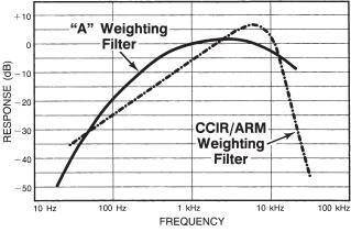
CCIR/ARM Weighting Filter (CCIR rec. 468-2, averageresponding meter, Dolby Labs Bulletin No. 19/4)
