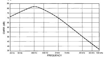
Typical CMRR: From 20 Hz to 100 kHz with input voltage of 6 volts.
