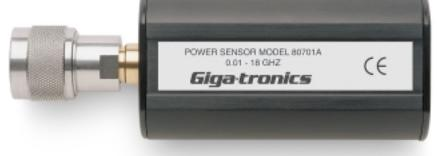
And the Giga-tronics 80701A Modulated Power Sensor operating with the 8650A power meter, provides system bandwidth up to 10 MHz to measure the peak and average power of wide band, third-generation CDMA signals over an 80 dB range.
