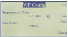
A volts per frequency input is available to set the cal factor when connected to an RF source. As the source frequency is modified the V/F output will automatically set the power meter to the correct cal factor, thereby eliminating the need for manual input.
