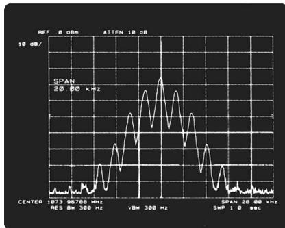
2. Second, press [FREQUENCY SPAN] and, using the data controls, reduce the, displayed frequency range.
