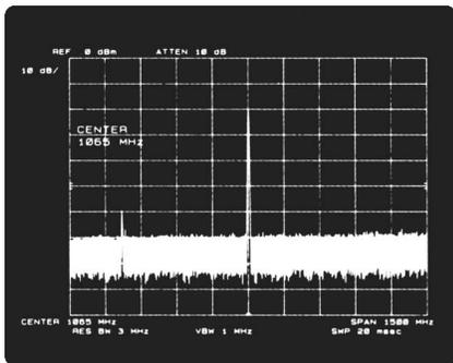
1. First, press [CENTER FREQUENCY] and position the signal at the center of the screen using one of the data controls (e.g., the knob, step keys, or the numeric keypad).
