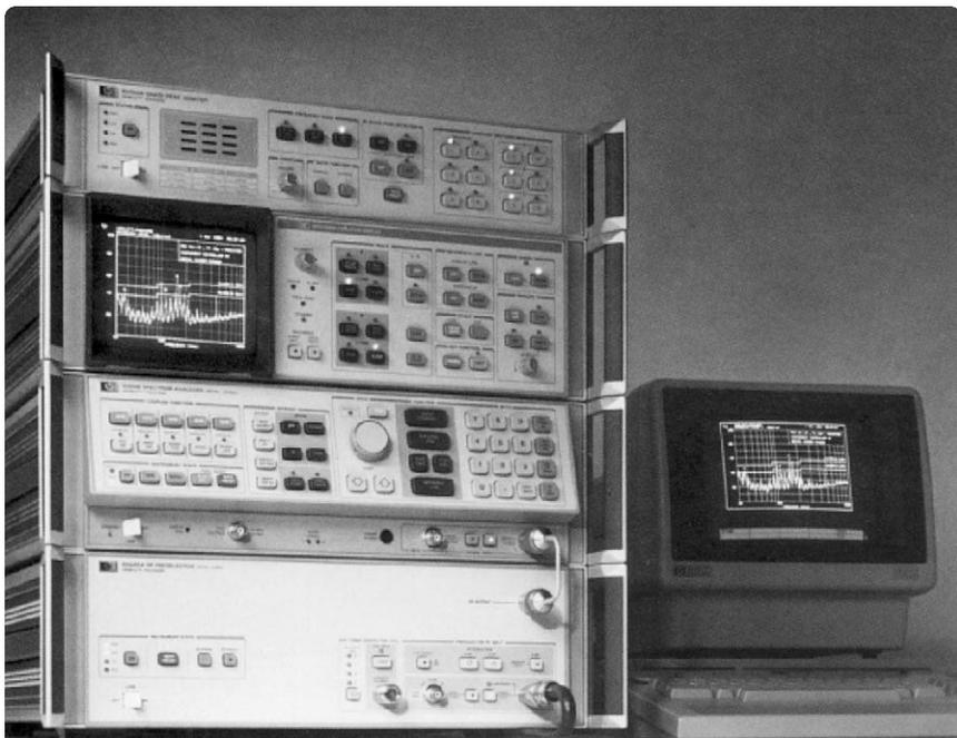
The spectrum analyzer has long been a useful tool in evaluating electromagnetic interference (EMI) spectra for troubleshooting and preliminary qualification testing. The 8568B spectrum analyzer, with high performance and full programmability, allows difficult and time-consuming EMI compliance tests to be completed automatically.
