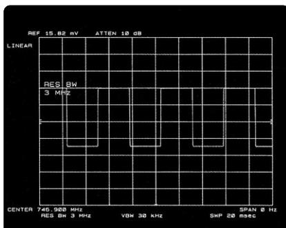
Wide 1 and 3 MHz bandwidths with "Gaussian" shapes improve sensitivity and transient behavior when measuring impulse noise, such as electromagnetic interference, or demodulating wideband spectra.
