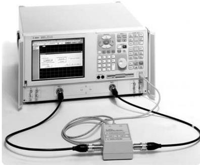
Calibration configuration using the PNA series
