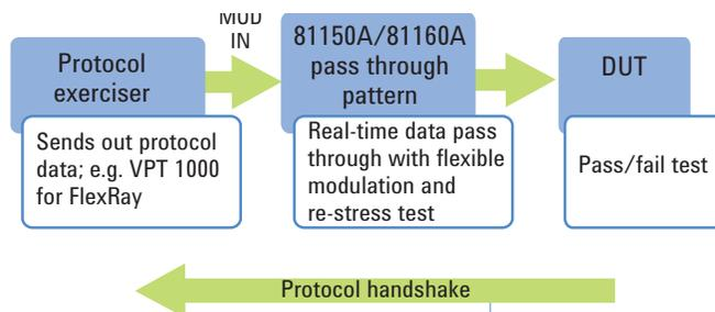
The pass-through pattern functionality takes the protocol data via “mod in” and adopts it to any kind of stress test (shape and timing changes).
