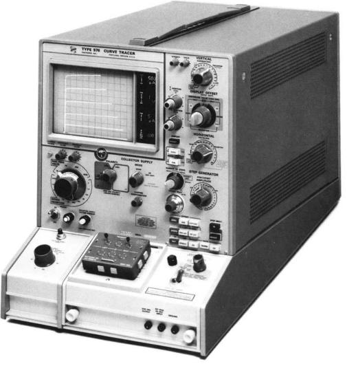
With the Standard Test Fixture, the collector supply of the 576 delivers up to 220 watts peak to the device under test. The step generator can deliver up to 2 amps in both its current and voltage modes of operation. With the 176 High-Current Fixture, the 576 is capable of pulsed collector operation up to 200 amps peak.
