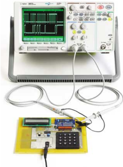
Figure 8. Trigger on address and/or data patterns within an I 2 C frame.
