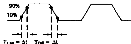
Measure transition times to 2 ns resolution with one push of a button.
