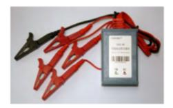
With proper number wireless modules, main tester can real time scan and display the voltage data of each battery during the discharging, and display the histogram of all batteries to follow the battery voltage tracks in whole discharging process.
