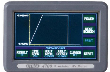
*Chart Mode automatically plots voltage readings from a few seconds to several days. Highly useful for determining ramp linearity, overshoot and sag on hipot testers and other HV sources.*
