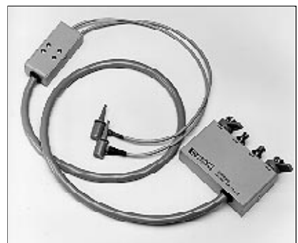
HP 16089C Kelvin IC Clip Leads IC package clip. 1 meter length.
