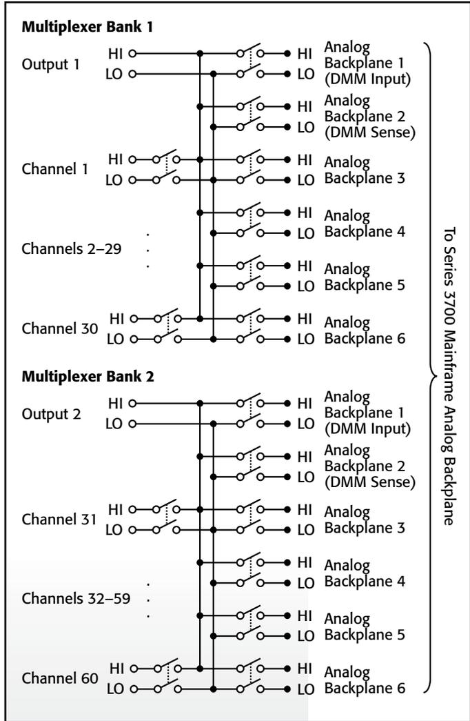
**MULTIPLEXER CONFIGURATION:** Two independent 1×30 2-pole multiplexers. Banks can be isolated from the backplane by relays. Card can be configured for 2 and 4 wire.
