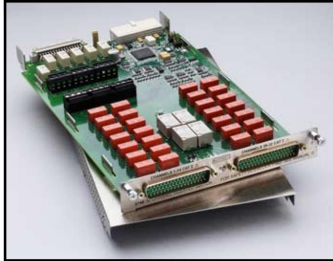
The Model 3740 offers 28 general-purpose form C channels that are ideal for routing power or other control devices. For higher power applications of up to 7A, four additional high current form A channels are provided.
