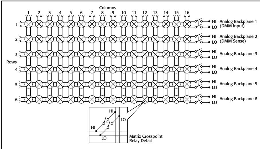
**MULTIPLEXER CONFIGURATION:** 6 row by 16 column matrix. Columns can be expanded using the backplane or isolated by relays.
