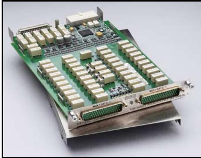
The Model 3721 offers two independent banks of 1×20 two-pole multiplexers that are ideal for general purpose switching, including temperature measurements. The two banks can automatically be connected to the Series 3700 mainframe backplane and optional DMM through the analog backplane connection relays. This connection allows the mainframe to reconfigure the Model 3721 as a single 1×40 two-pole multiplexer or to enable card-to-card expansion for even larger configurations.
