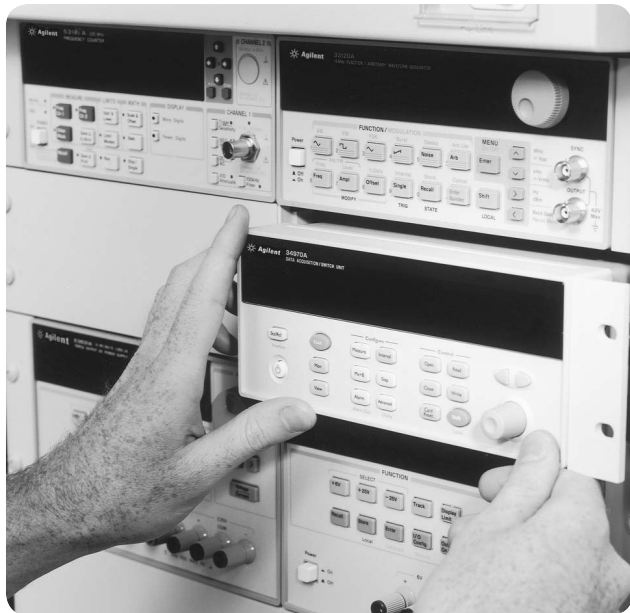
Low-cost switching system for automated testing
