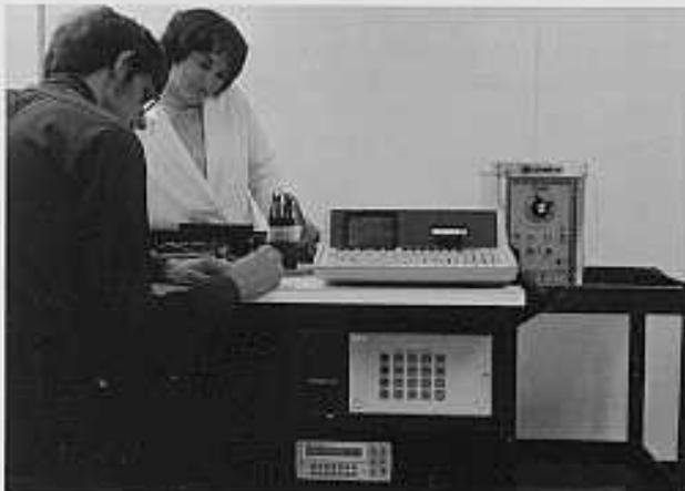
Production testing of temperature probes.
