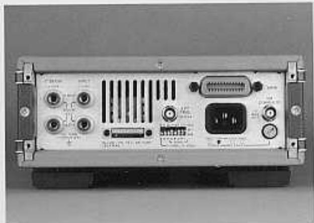
Switchable rear inputs and synchronizing signals.
