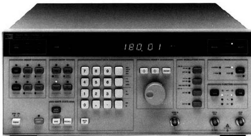
The HP 3326A Two-Channel Synthesizer combines two independent synthesizers, flexible modulation, and control circuitry into a single, powerful package. This single instrument can provide precise phase offset, two-tone sweep, fast frequency switching, internal modulation, and pulse signals for bench or systems use.
