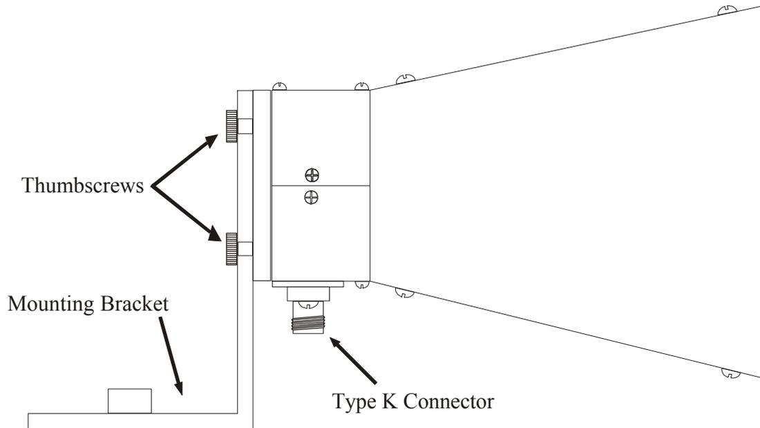
*NOTE This illustration shows the Model 3116 vertically polarized for the purpose of introducing the primary mounting components. Typically the horn will be mounted in the horizontally polarized position for testing.*
