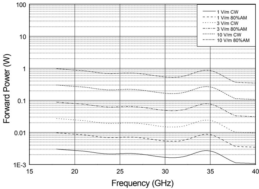
Model 3116 Forward Power at 1 meter 1V/m to 10 V/m
