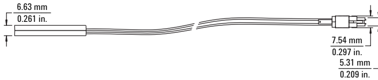
Figure 3.6. E5394A and E5396A soft touch probe dimensions
