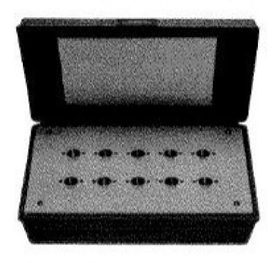
Calibration standard for performance testing and adjustment of the 4193A. Includes ten probe-insertable standards: OPEN, SHORT,  $10\Omega$ ,  $50\Omega$ ,  $100\Omega$ ,  $180\Omega$ ,  $1k\Omega$ ,  $1.8k\Omega$ ,  $10k\Omega$ , and 5pF. If a standard is damaged or fails to perform properly, contact your nearest Hewlett-Packard Sales and Service Office.
