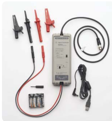
N2791A 25 MHz high voltage differential probe
