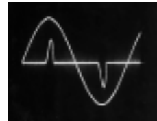
Same conditions with programmable Z^{\circ} engaged. THD=0.25%
