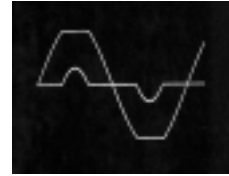
Oscillograph of voltage and current waveform at load due to distribution losses. THD=6.6%
