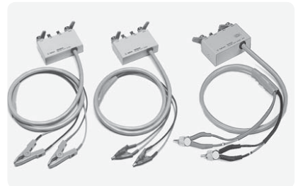
16089A/B/C/D/E clip leads Connector type: A/B/C/E: Kelvin D: alligator Frequency: 5 Hz to 100 kHz Cable length: A/B/C/D: 0.94 m E: 1.3 m
