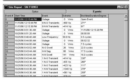
Homes, offices, hospitals, and factories depend on electronic devices. And electronic devices depend on good power quality. The Fluke VR101S is the perfect system for catching sags, swells, transients, outages and frequency variations on line voltage at receptacles, where the most sensitive loads are connected.
