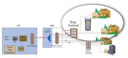
The PPM-350B allows for pass-through connection in any PON architecture.
